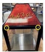
Remove (2) screws from the bracket in which the temp. sensor runs under; remove the bracket.
