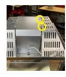
Remove the nut holding the temp. sensor in place; remove temp. sensor. Using the new sensor, complete all steps in reverse order & you have successfully replaced your units temperature sensor.
