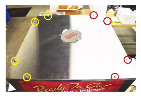
Remove side panel by pushing the graphic panel in gently to separate the latches. Then pull the panel up and out.
