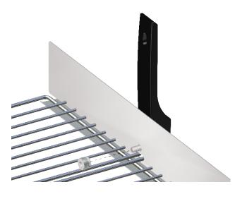
5 Thread and tighten the Thumb Nut onto the Screw
