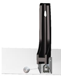
Insert the Screw through the Grill Loop, the Handle Bracket, and the Grill Front
